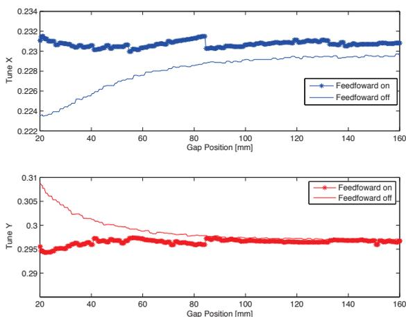
Figure 3: The measurement tune when U58 gap varies.
