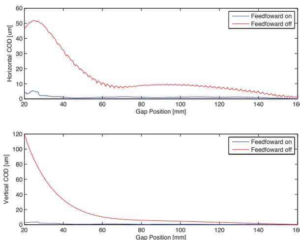
Figure 2: The CODs in both planes before and after correction during gap variation.
