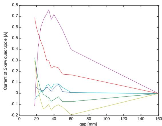
Figure 8: Skew quadrupole settings for coupling correction.
