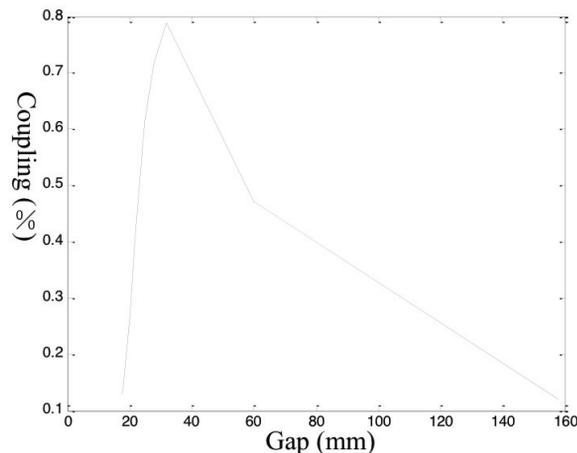
Figure 7: the coupling varies when gap changes.
