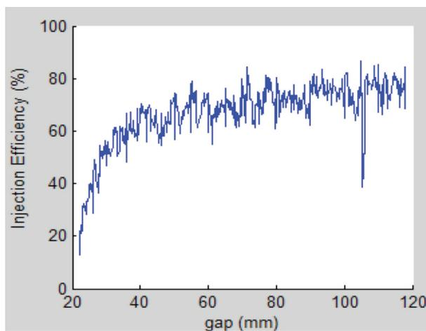
Figure 5: injection efficiency when the gap changes.
