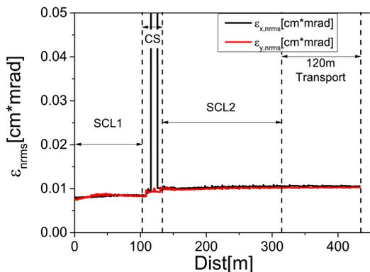
Figure 5: Normalized RMS emittance of Uranium in RAON main driver linac.
