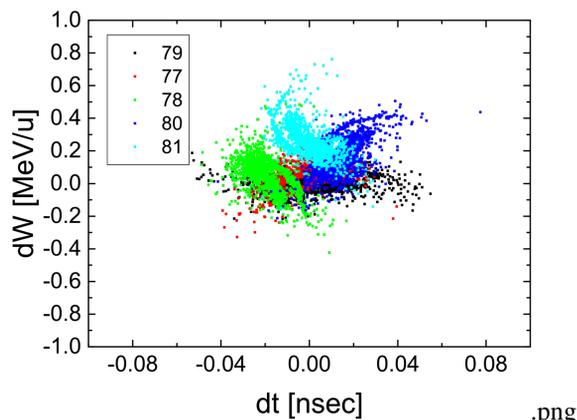
(c) Beam profile in longitudinal phase space
