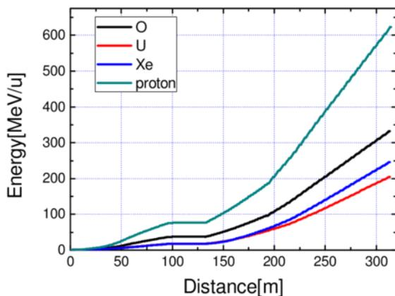
Figure 3: Ion energies in SCL.
