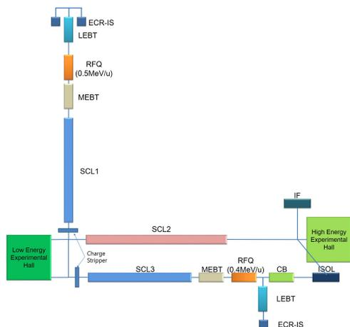
Figure 1: Layout of RAON superconducting linacs.
