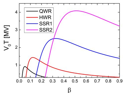
Figure 2: Effective accelerating voltage of cavities in RAON superconducting linac.
