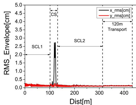
Figure 4: RMS envelope of Uranium in RAON main driver linac
