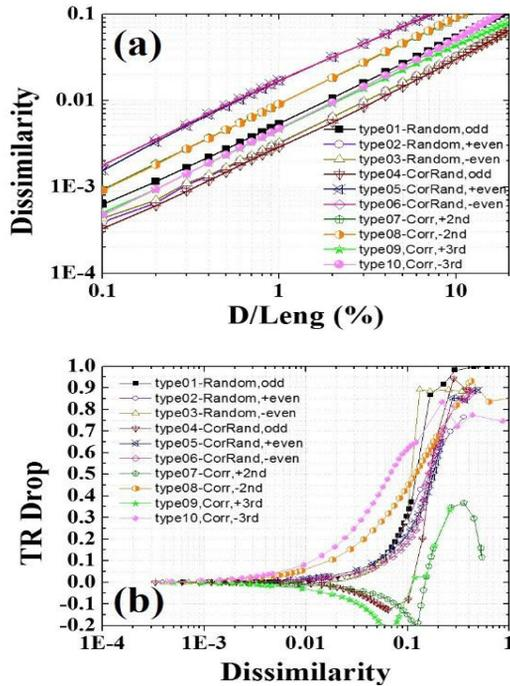
Figure 3: The relation between the deformation parameter and the dissimilarity (a). The relation between the dissimilarity and the TR drop (b). The TR drop is the ratio of the deviation of TR to the original value.
