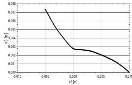
Figure 4: The typical mask shape to generate a triangle current profile. This shape shows positive y-side only. The shape is vertically symmetric.
