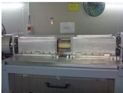
Figure 1: Vertical (left) and horizontal (right) pinger magnet installed at ALBA during summer 2014. The ceramic chamber (in white) is visible between the two structures used for the vertical (left) and horizontal (right) excitations.
