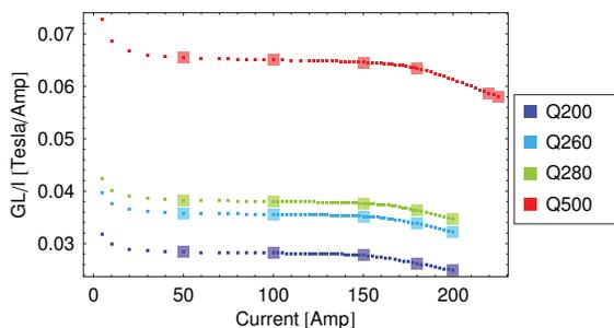
Figure 1: Integrated gradient normalized to the excitation current as a function of the current setpoint for each type of ALBA SR quadrupole. Large symbols stand for the original data provided by the manufacturer, and small symbols correspond to the detailed measurements carried out at ALBA.
