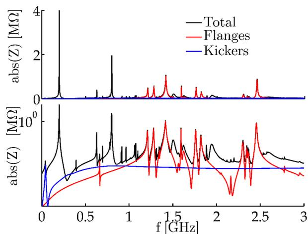
Figure 1: Modulus of the current longitudinal impedance of the SPS. The red and blue traces show the contribution of the vacuum flanges and the kickers, respectively. The top and bottom plots show the impedance in linear and logarithmic scale, respectively.
