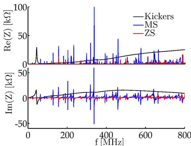
Figure 2: Real and imaginary parts of the longitudinal impedance of 25 MS and 5 ZS compared to the total longitudinal kicker impedance.
