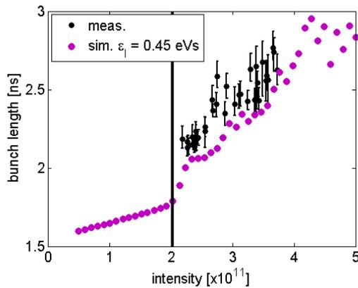
Figure 3: Measured and simulated bunch length as a function of intensity for a single bunch at the SPS flat top in a double RF system (bunch shortening mode). The voltage at 200 MHz was 2 MV and at 800 MHz 200 kV.
