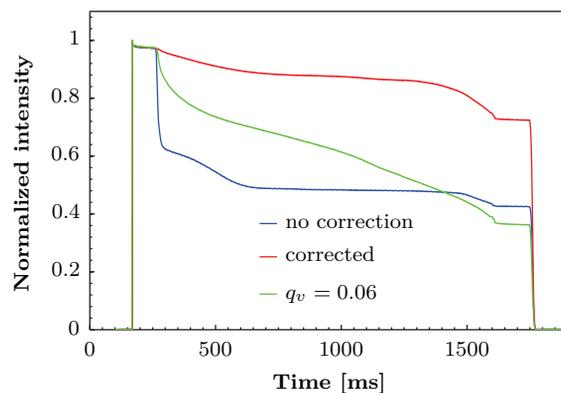
Figure 4: Influence of orbit correction on beam loss. For the blue and red curves the vertical tune was programmed to 6.10. With an active correction the vertical tune could be programmed closer to the integer resonance (green curve), which was impossible without correction.
