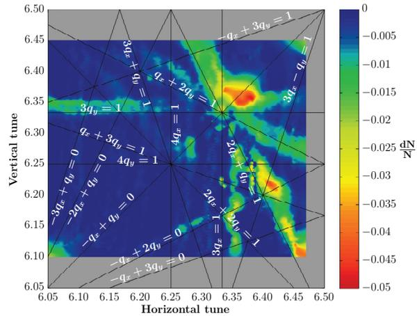
(b) Vertical scan from top to bottom conducted before the realignment. Beam loss along the vertical line  $Q_x = 6.35$  corresponds to an interpolation artifact.
