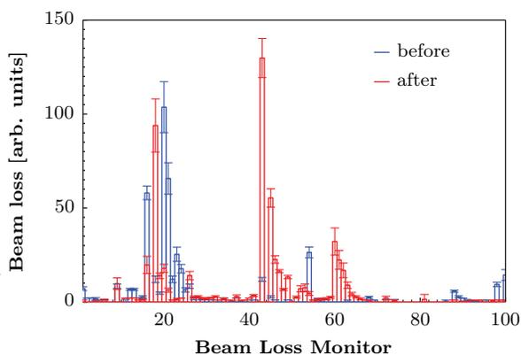
Figure 3: Comparison of loss patterns before and after the realignment measured with the BLMs. The same machine settings as in Fig. 2 were applied, and the accumulated losses at the end of the measurement cycle are depicted. The error bars represent the standard deviation calculated using three recorded data sets.
