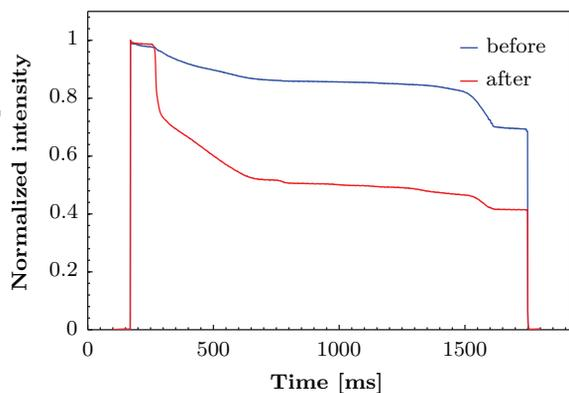
Figure 2: Comparison between intensity profiles before and after the realignment for programmed vertical tunes of 6.10. The horizontal tune is dynamically changed from 260 ms onwards, which corresponds to the drastic drop of the intensity.
