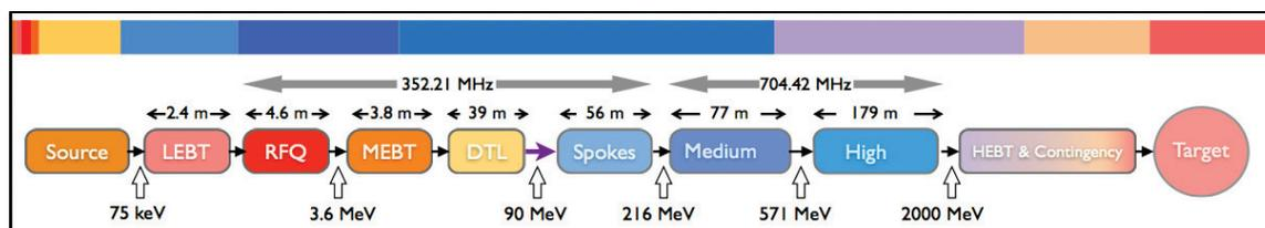
Figure 1: Schematic block diagram of the ESS accelerator lattice (bottom) and corresponding proportional length of the different sections (top). The blue items are superconducting (i.e. the spoke resonators, the medium and high  $\beta$  elliptical cavities), while the other items are normal conducting.
