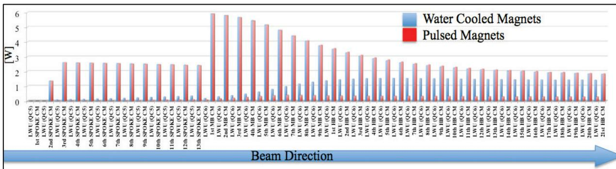
Figure 4: Integrated power on beam elements from the first spoke until the last high- $\beta$  cryomodules. For the LWUs the shown values are the sum of the power in the two magnets (i.e. yokes plus coils), excluding the beam-pipe and the LWU support. Errors are less than 1%. FLUKA results about the cryomodules are of the same order of those found with MARS ones [11].
