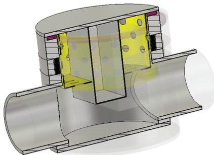
Figure 3: The Shielded RP has been designed to optimize the impedance of the box RP without a complete redesign.
