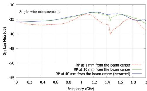
Figure 9: Transmission coefficient ( $S_{21}$ ) for the wire test with the Cylindrical RP at 1 mm, 10 mm and 40 mm from the center of the beam pipe.
