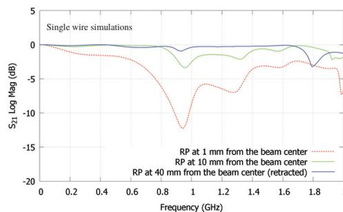
Figure 10: Simulated transmission coefficient ( $S_{21}$ ) for the wire test with the Shielded RP at 1 mm, 10 mm and 40 mm from the center of the beam pipe.
