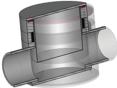
Figure 2: The Cylindrical RP has been designed to increase the space available for the detector and to decrease the impedance.
