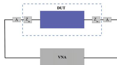
Figure 6: A single wire is stretched along the device under test (DUT) and connected to a Vector Network Analyzer (VNA). The impedance matching is ensured by the network (block “ $Z_m$ ”) and the series attenuator (block “A”).
