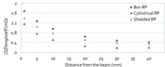
Figure 5: The cylindrical RP has a  $\sim 50\%$  better  $(\Im Z_{long}/h)^{eff}$  than the box RP at 1 mm from the beam.
