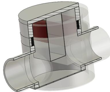
Figure 1: Before LS1 all Totem Roman Pots were box shaped. The empty space between the RP and the flange resonate at low frequency ( $\sim 500$  MHz).
