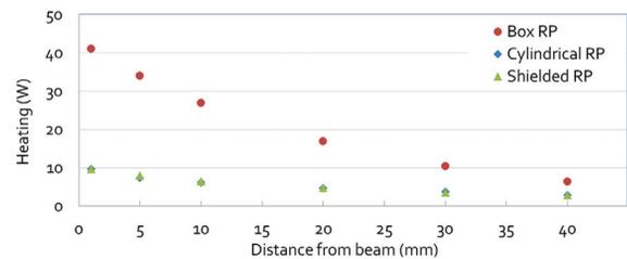
Figure 4: The cylindrical and the shielded RPs have a  $\sim 4$  times lower heating than the box RP at 1 mm from the beam, with a 25ns beam spacing, 2800 bunches and  $1.310^{11}$  protons per bunch (beam current of 0.65A).
