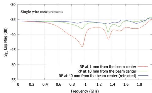
Figure 11: Transmission coefficient ( $S_{21}$ ) for the wire test with the Shielded RP at 1 mm, 10 mm and 40 mm from the center of the beam pipe.
