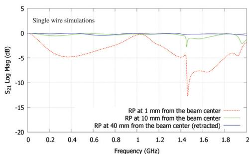
Figure 8: Simulated transmission coefficient ( $S_{21}$ ) for the wire test with the Cylindrical RP at 1 mm, 10 mm and 40 mm from the center of the beam pipe.
