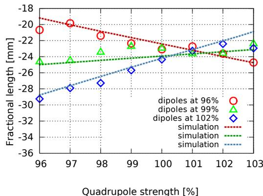
Figure 4: Ring length measured as function of the quadrupole strengths with the dipoles fixed at different values.
