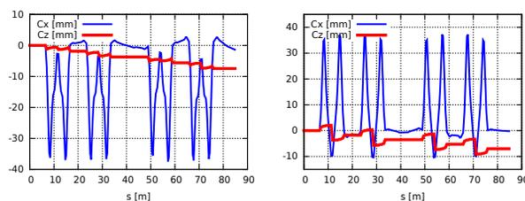
Figure 1: Horizontal and longitudinal bunch position computed for one turn in the combiner ring for two different scalings of the optics: left Q@95%, D@105%; right Q@105%, D@95%.
