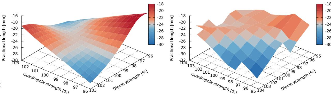
Figure 6: Responses of the CTF3 combiner ring length to quadrupole and dipole strengths variations. Left: PLACET2 simulations. Right: measured data.
