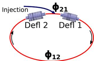
Figure 7: Scheme of the notation used:  $\phi_{21}$  is the phase advance over the injection septum, while  $\phi_{12}$  represent the phase advance in the complementary part of the ring.
