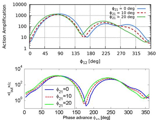
Figure 8: Action amplification due to the long-range wakefields as function of the phase  $\phi_{21}$  computed with PLACET2 (top) and by D. Alesini (bottom).
