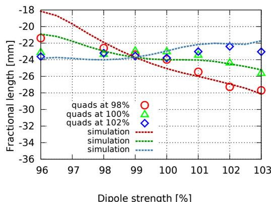
Figure 5: Ring length measured as function of the dipole strengths with the quadrupoles fixed at different values.
