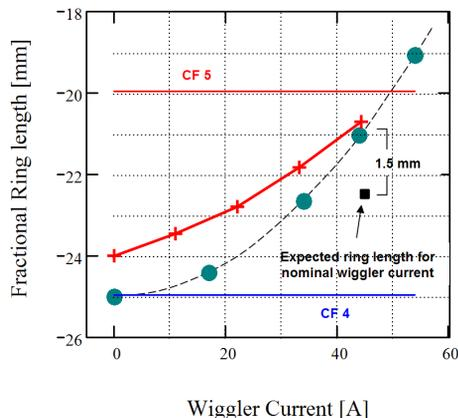
Figure 3: Effect of the wiggler current on the ring length. The red crosses are the new measurements, the blue dots are found in [4].
