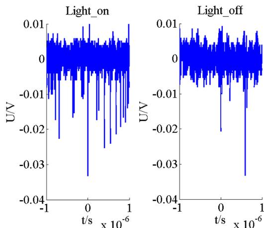
Figure 3: Signals detected in the lab, with ambient light off (right) and on (left).
