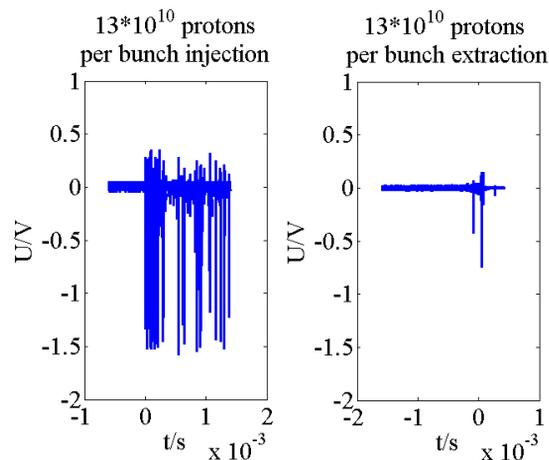
Figure 4: Signal in the photon detector with closed aperture: just after injection (left) and just before extraction (right). The zero of the abscissa correspond to the injection and extraction time, respectively.
