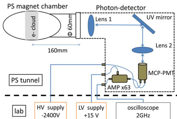
Figure 2: Schematic setup of the detector in the PS.
