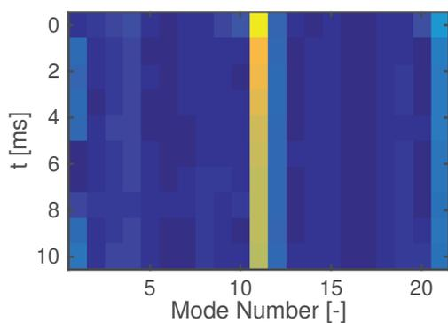
Figure 3: Mode amplitude evolution in  $h = 21$  and 21 bunches. One unstable mode ( $i=11$ ,  $\mu=10$ ) is visible.
