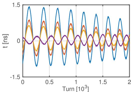
Figure 2: Plot of center of mass oscillation of 4 bunches in the case of  $n_b = 18$  in  $h = 21$ .
