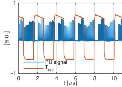
Figure 1: Longitudinal PU signal (WCM95) and beam synchronous  $T_{rev}$  signal (it is a signal proportional to the harmonic of the machine) acquired during measurements.
