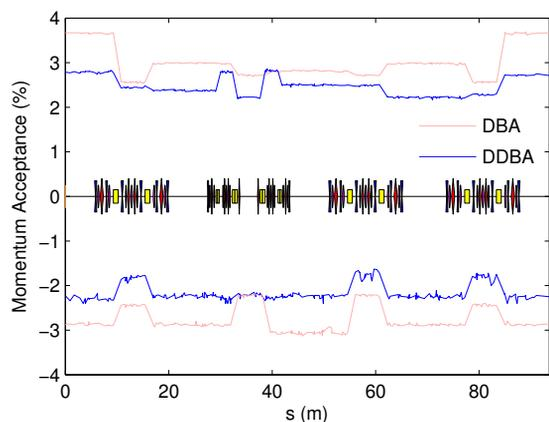
Figure 4: Momentum aperture for one super-period of the existing and upgraded rings in low alpha optics.
