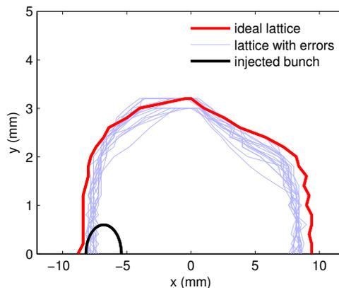
Figure 5: On-momentum dynamic aperture over 25 error seeds. The injected beam area for  $2\sigma_x \times 2\sigma_y$  is highlighted for clarity.
