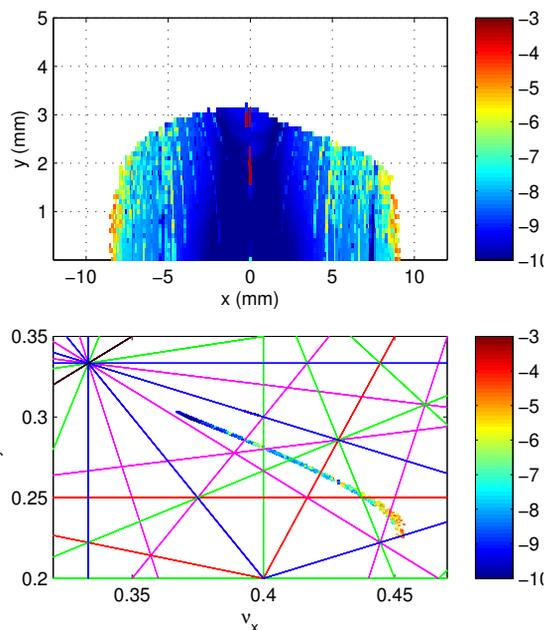
Figure 3: Dynamic aperture (top) and frequency map (bottom) for the low alpha lattice.
