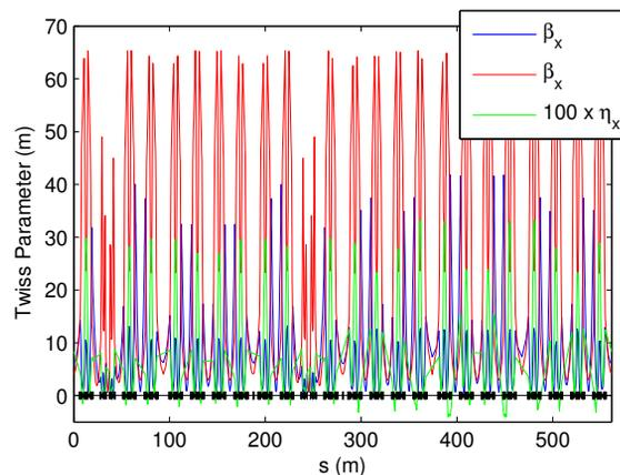
Figure 6: Twiss parameters for the present two-DDBA lattice solution for low alpha optics.
