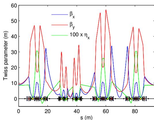
Figure 2: Twiss functions for the DDBA lattice in low alpha mode.
