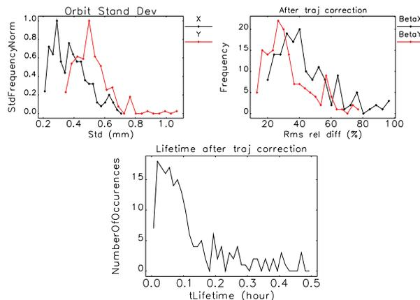
Figure 1: Top left: Distribution of standard deviation of orbit after trajectory correction calculated over 200 random error seeds. Top right: Distribution of rms relative beta function errors after trajectory correction. Bottom: Lifetime after trajectory correction for 1-mA bunch.
