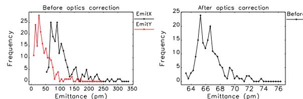
Figure 4: Left: Distribution of horizontal and vertical emittances after orbit correction (before lattice correction). Right: Horizontal emittance after lattice correction.
