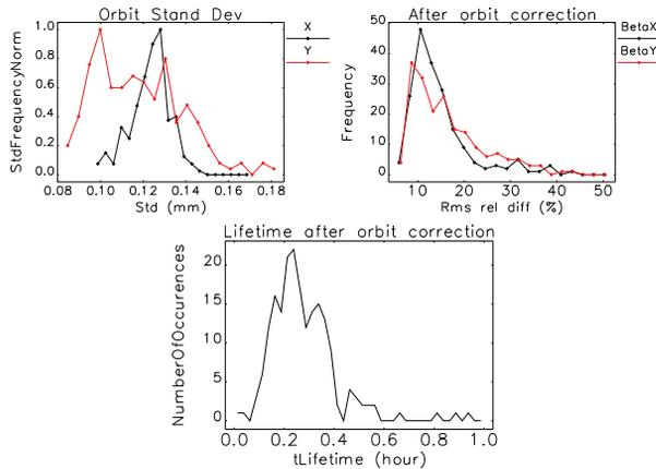
Figure 2: Top left: Distribution of standard deviation of orbit after correction calculated over 200 random error seeds. Top right: Distribution of rms relative beta function errors after orbit correction. Bottom: Lifetime after orbit correction for 1-mA bunch.
