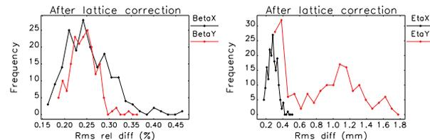
Figure 3: Left: Distribution of rms relative beta function errors after lattice correction. Right: Rms errors of the dispersion after lattice correction.
