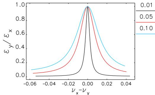
Figure 3: Calculated beam respect ratio ( $\varepsilon_y/\varepsilon_x$ ) vs. tune separation ( $\nu_x - \nu_y$ ) at different coupling  $\kappa$  (legend) for APS.
