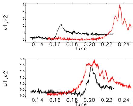
Figure 4: Measured tune spectrum at normal operational tunes (top) and at coupling resonance (bottom).
