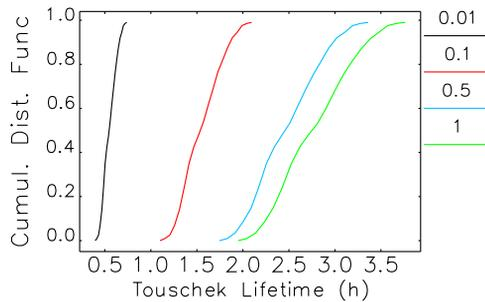
Figure 1: Cumulative distribution functions for the Touschek lifetime from the 100 error ensembles of H7BA optics at different emittance ratios (legend).
