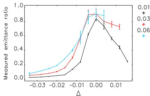
Figure 7: Calculated beam aspect ratio ( $\epsilon_y/\epsilon_x$ ) vs. tune separation  $\Delta$  at different  $\kappa$  (legend). The measured  $\Delta$  range for  $\epsilon_y/\epsilon_x \leq 0.8$  is about 0.01 for  $\kappa = 0.03$ .
