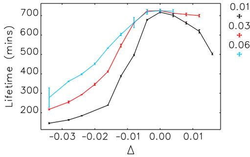
Figure 6: Measured beam lifetime (fitted over 1 min) vs. tune separation  $\Delta$  at different  $\kappa$  (legend).
