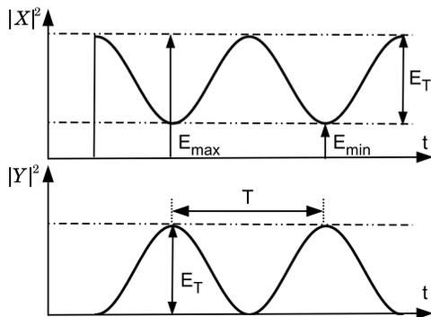
Figure 2: Behavior of the envelope functions of the coherent oscillations following a kick in one plane.
