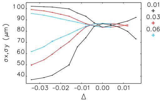
Figure 5: Measured beam size (raw data) and coupling vs. tune separation  $\Delta$  at different  $\kappa$  (legend).
