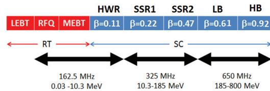
Figure 2: Technology map of PIP-II linac.
