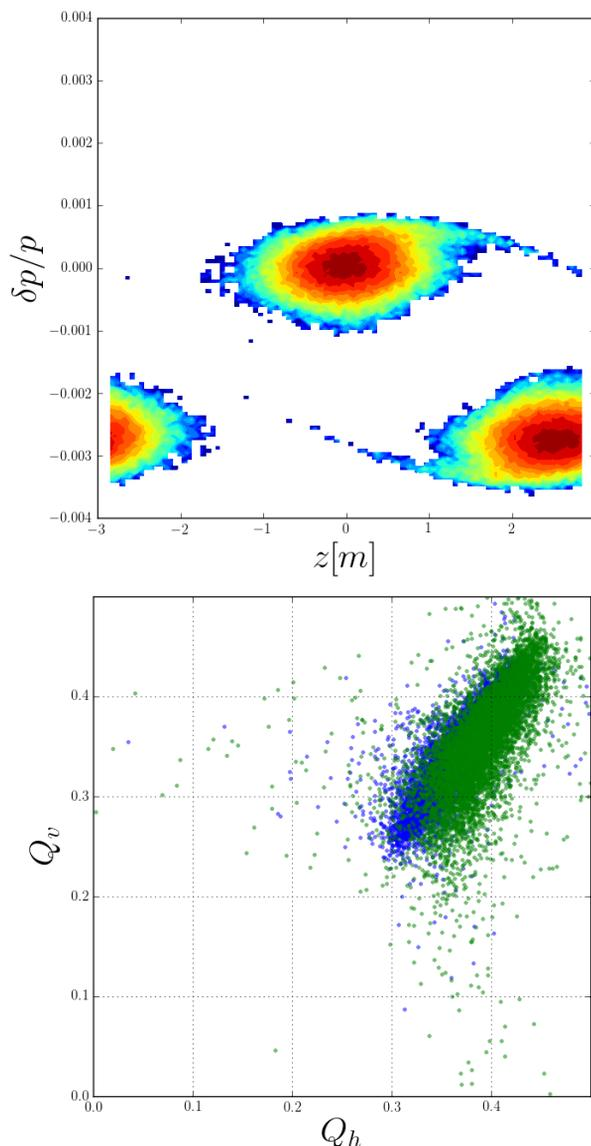
Figure 2: Upper: longitudinal phase space of two bunches close to maximum separation. Lower: tune footprint of the upper momentum (blue) and lower momentum (green) bunches. The lower momentum bunch is slipping to the right.
