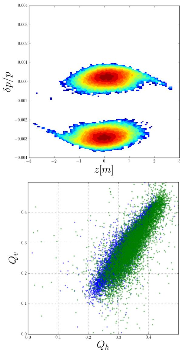
Figure 3: Upper: longitudinal phase space of two bunches close to full spatial overlap. Lower: tune footprint of the upper momentum (blue) and lower momentum (green) bunches.
