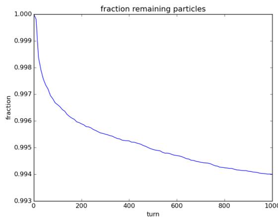
Figure 4: Fraction of particles remaining as a function of turn with vertical restriction.
