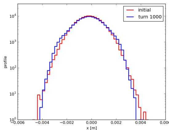
Figure 5: Effect of the vertical restriction on the horizontal particle distribution. The initial horizontal particle distribution is shown in red, and after 1000 turns is shown in blue.
