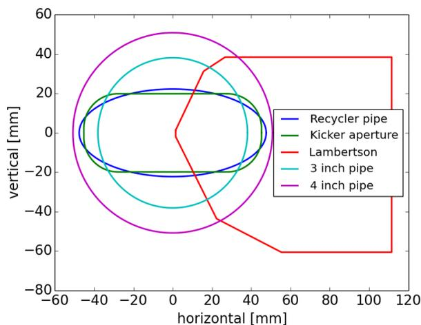
Figure 1: Apertures in the Recycler.
