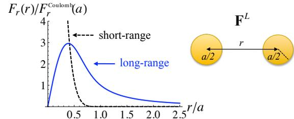
Figure 1: Short-range and long-range contributions to the Coulomb force between two particles (1) for a given cutoff radius  $a$  used by a P<sup>3</sup>M solver in IMPACT-T.
