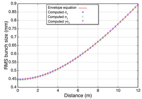
Figure 2: RMS beam sizes  $\sigma_x$ ,  $\sigma_y$ , and  $\gamma\sigma_z$  as functions of drift distance for a 0.25 nC electron bunch expanding in free space at 250 MeV, for comparison with (2). Results are obtained using a P<sup>3</sup>M solver with  $a/H = 3$ .
