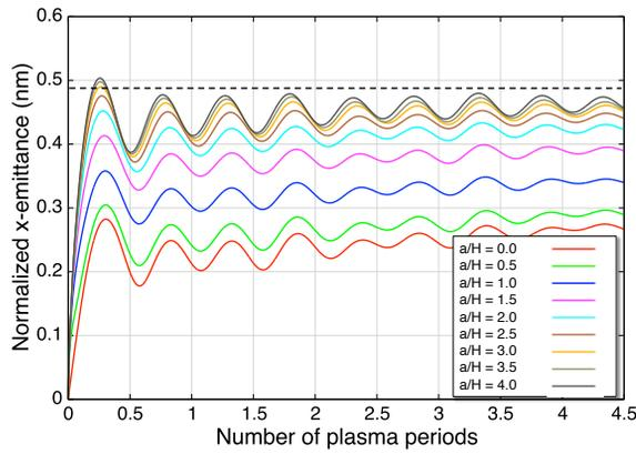
Figure 4: Emittance growth of a confined 25 fC electron bunch undergoing disorder-induced heating as obtained using a P<sup>3</sup>M solver. Results are shown for several values of the cutoff radius  $a$ .
