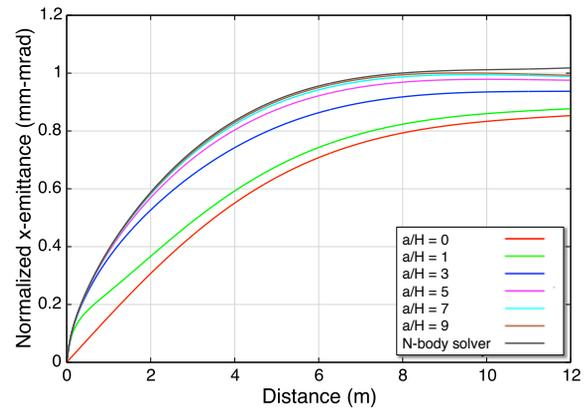
Figure 3: RMS horizontal emittance of a 0.25 nC electron bunch expanding in free space at 250 MeV as obtained using a particle-in-cell solver (red), a direct N-body solver (black), and a P<sup>3</sup>M solver with cutoff radii  $a/H = 1, 3, 5, 7$ , and 9.
