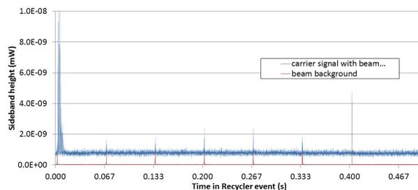
Figure 3: Second microwave measurement. Spectral power of the lower sideband frequency averaged over 40 Recycler cycles and for each of two cases - with the carrier signal and without.
