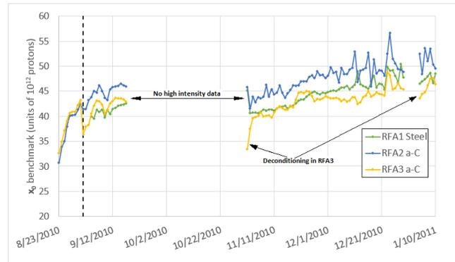
Figure 6: The daily fit of the  $x_0$  benchmark is shown over time for RFA1 (steel), RFA2 (a-C near steel), and RFA3 (a-C). After a vacuum leak occurs (dashed line) near to RFA3, the  $x_0$  benchmark for RFA3 decreases dramatically and lags behind RFA2.
