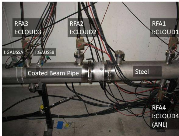
Figure 5: The electron cloud measurement setup in the Main Injector at MI-52. The setup primarily consists of four RFAs and two beampipe sections. The beampipe is 6" in diameter and the coated and uncoated sections are each ~1 meter long. The setup is located in a straight section to avoid electron confinement from magnets.
