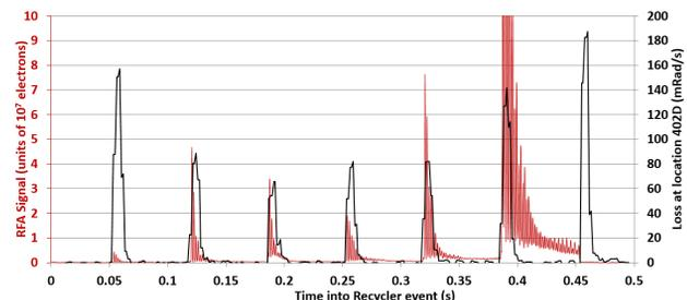
Figure 4: Signals from an RFA (red) measured in volts and a typical loss monitor (black) over the Recycler cycle.
