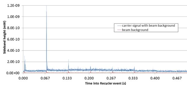
Figure 2: First microwave measurement. Spectral power of the lower sideband frequency averaged over 40 Recycler cycles and for each of two cases - with the carrier signal and without.
