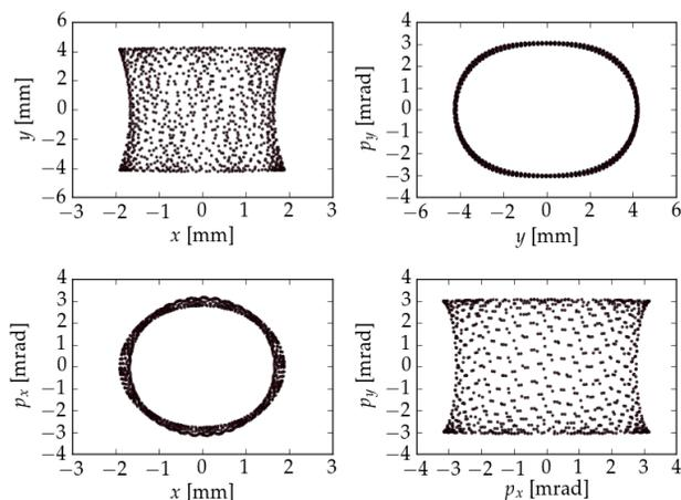
Figure 4: Poincaré sections for the transverse particle dynamics.
