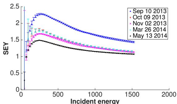
Figure 2: SS316L SEY measurements during 2013-2014.
