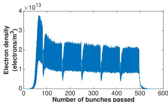
Figure 9: Electron cloud density within one sigma of the proton beam.
