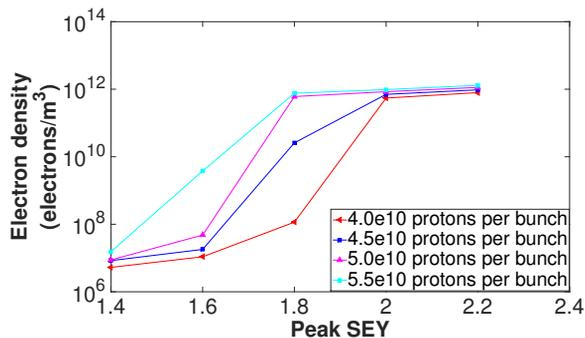
Figure 5: Maximum electron density vs. peak SEY at different beam intensities.
