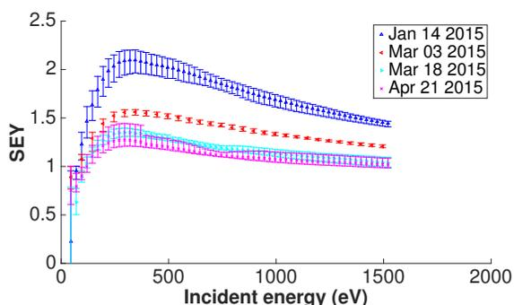
Figure 3: TiN coated SS316L SEY measurements.
