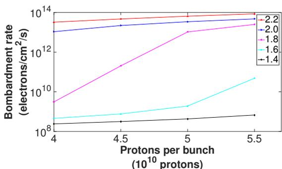
Figure 6: Simulation of bombardment rate on the vacuum chamber with different peak SEY.
