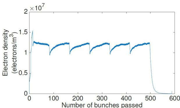
Figure 7: Electron cloud density for peak SEY 1.4 and  $4.0e10$  protons per bunch.
