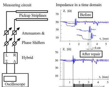
Figure 3: Schematic draw of the measuring circuit for head-tail modes observation experiment (left figure) and impedance in a time domain of pickup striplines before and after repair (right column of figures).
