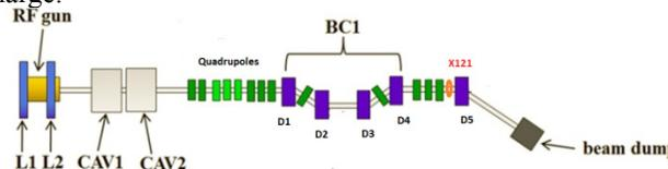
Figure 1: The 50 MeV electron beamline showing the RF gun followed by CAV1 and CAV2 that will accelerate the beam to 50 MeV. The green boxes show the quadrupoles used to focus the beam. The purple boxes are the dipoles that are used to bend the electron beam. D5 is the spectrometer dipole that is used in measuring the energy spectrum of the bunch. X121 is an Optical Transition Radiation (OTR) monitor that will be used to measure the current profile of the electron beam [11].
