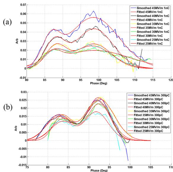
Figure 3a-b: Gun phase measurements for 1 nC bunch (a) and 300 pC bunch (b) collected using the faraday cup diagnostic for different gun gradients ranging from 25 MV/m to 45 MV/m (corresponding to beam energies of 2.5 MeV to 4.8 MeV). One degree corresponds to 2.14 ps for the L-band photoinjector.
