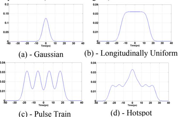
Figure 2a-d: (a) – Incoming gaussian laser pulse. (b) – Calculation of a longitudinally uniform laser pulse using three crystals with lengths (4.5, 9 and 18 mm). (c) – Calculation of a four pulse train using two crystals with lengths (13.3 and 27 mm). (d) – Calculation of a hotspot using three crystals with lengths (9, 18 and 25 mm).
