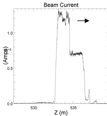
Figure 5: Beam current at turn 45, at a compression rate of 1.0 ns/turn.
