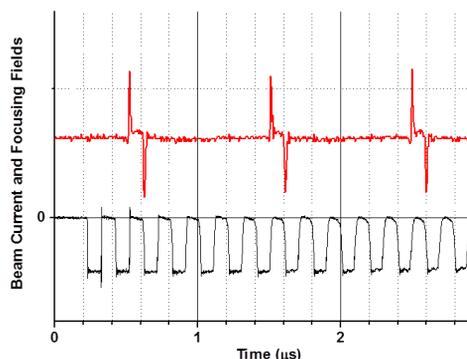
Figure 1: Synchronization between the barrier bucket fields (red) and beam current (black) from the wall-current monitor in the ring.
