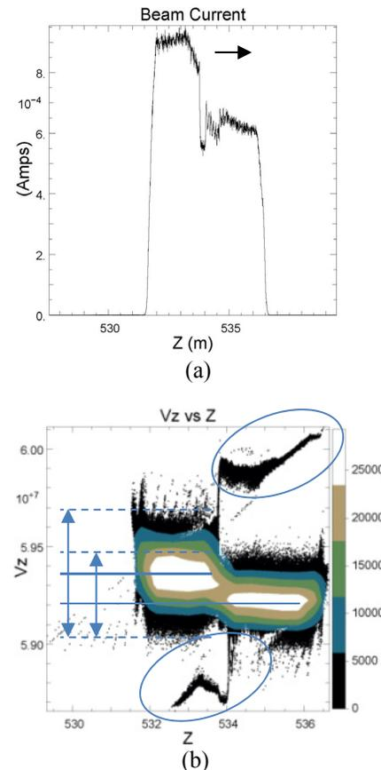
Figure 4a-b: (a) – Beam current at turn 45, at a compression rate of 0.5 ns/turn. (b) – Longitudinal ( $v_z$ - $z$ ) phase-space at the same compression rate.
