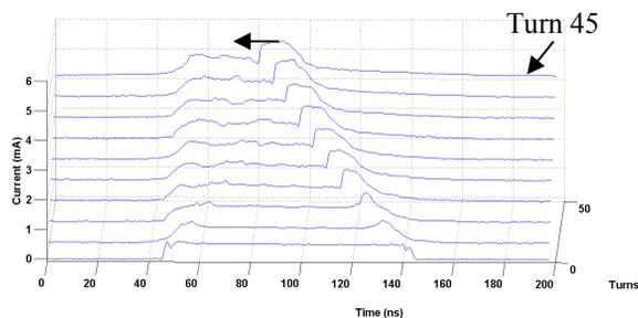
Figure 3: Beam current with compression at a rate of 1.0 ns/turn
