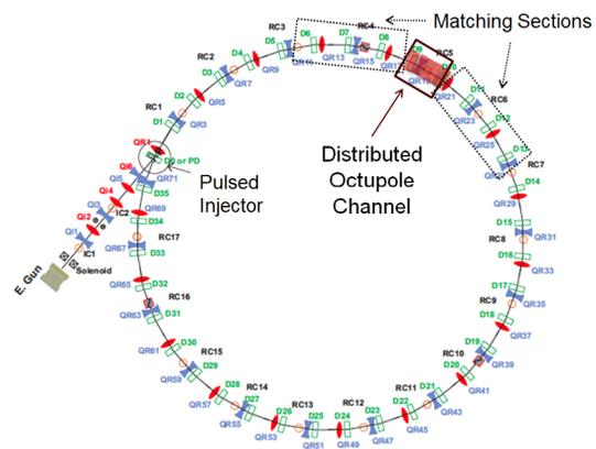
Figure 2: UMER lattice showing quadrupole and dipole elements, with overlay of future octupole channel.
