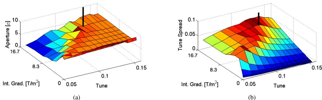
Figure 4: Parameter space landscape of toy octupole lattice, generated with Elegant FMA for 1024 turns. (a) Dynamic aperture and (b) Maximum tunespread vs. integrated octupole strength and lattice tune.
