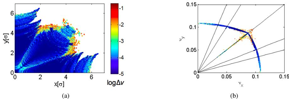
Figure 3: Frequency map analysis (FMA) of toy octupole lattice in WARP PIC code. (a) Change in tune vs. particle launch position. (b) Tune footprint, with 1st to 3rd order resonance lines.
