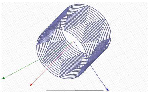
Figure 5: Preliminary single-layer printed circuit octupole design in Maxwell 3D.
