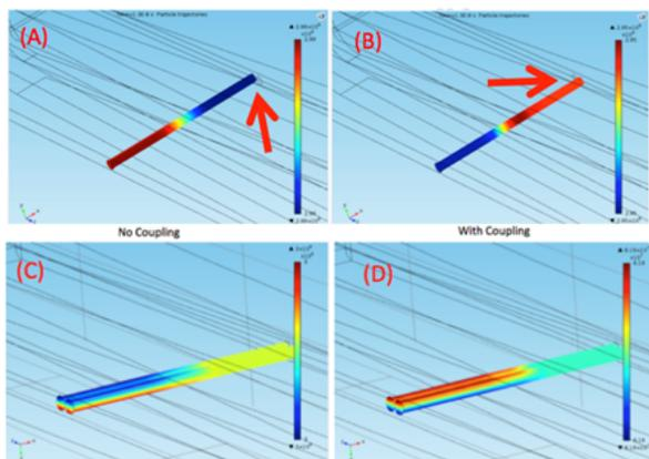
Figure 6: (A) Turn N injected bunch to the RF cavity, (B) turn N+1 bunch, (C) two bunches do not couple in the cavity, (D) two bunches couple via Wakefield.
