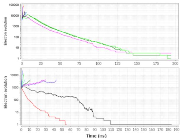
Figure 4: The surface phenomenon on the Bellows, or corrugations, is purely corona as the electron multiplication does not meet multipacting signature. As the electron count is doubled, the electrons impacted with increasing power insertion does not scale appropriately to indicate multipacting. The above shows multipacting at 40 dB at a simplified port-coupler location. Coupler is not centred correctly in the design.
