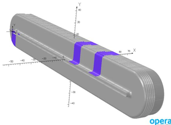
Figure 2: SFC straight cavity is designed from many sections. E&M calculations are made of parts for meshing. Matching of meshes initially introduced larger than normal corona at the seams. We fixed these problems as shown in Figure 4a.
