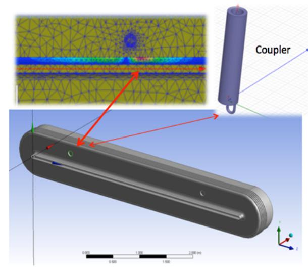
Figure 5: SFC cavity has shown resilience to pondromotive forces by producing clean S12 transfer function. Further studies of next generation cavity for a 100 MeV SFC require more rigorous work as reshaping the cavity produces RF field leakage and asymmetry which are not present in this cavity.
