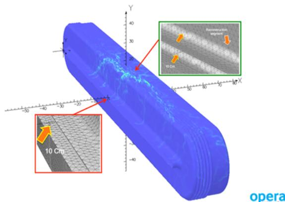
Figure 3: SFC straight cavity shows corona and not multipacting after further studies of E&M. The rate of Corona and its signature does not match the multipacting of 4a at high power due to primitive coupler design. The location of the coupler will be altered to determine its effects in future calculations.
