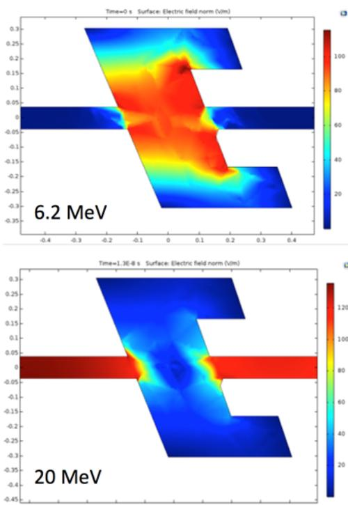
Figure 7: Wakefield effect of leading turn bunch is on trailing one is shown.
