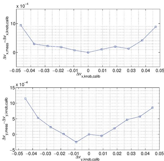
Figure 2: The residual tune variations after applying the tune knob calibrations.
