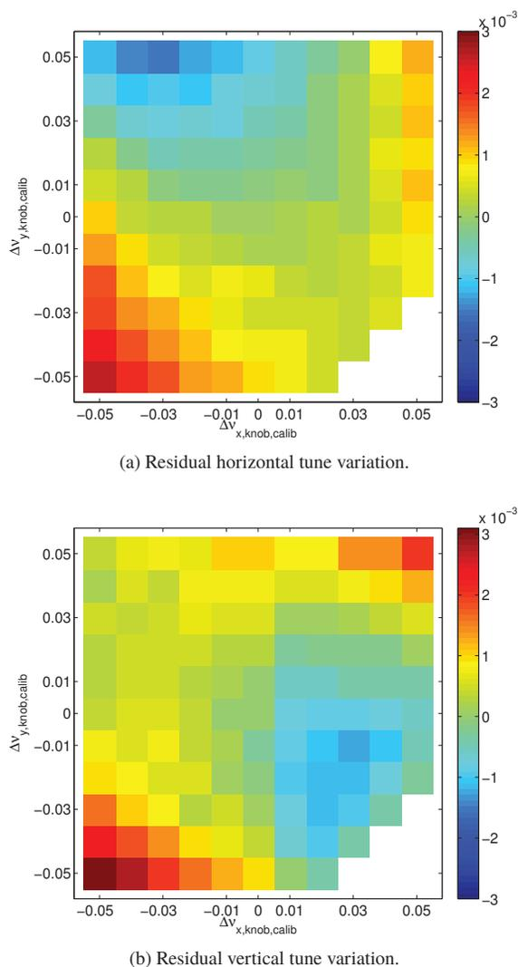
Figure 3: Residual tune variations by varying the horizontal and vertical tune knobs simultaneously.
