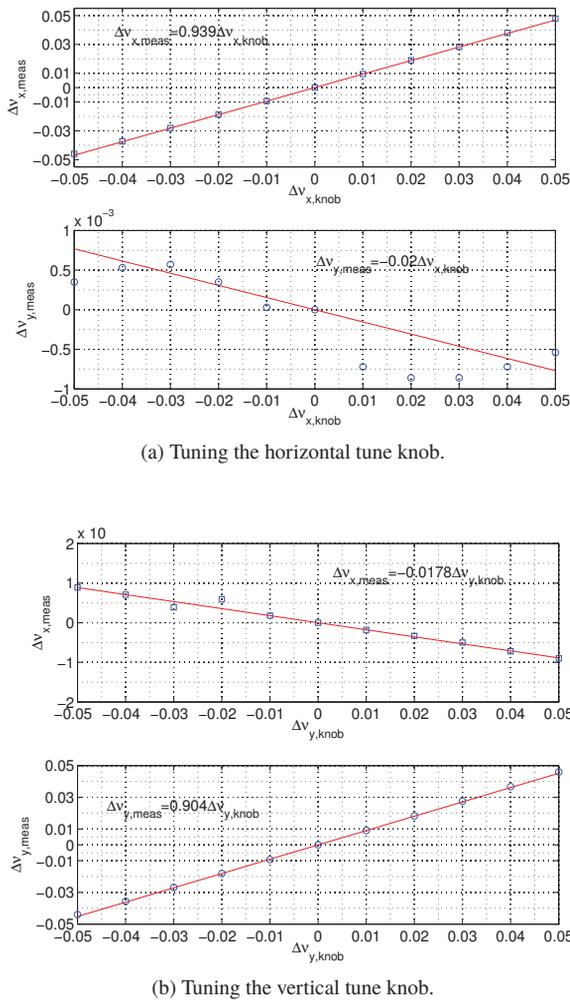
Figure 1: Measured horizontal and vertical tune variations by varying the tune knobs.
