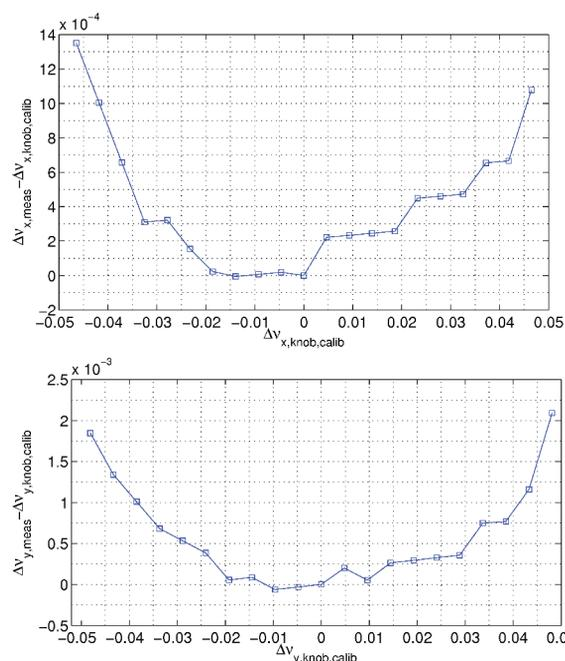
Figure 4: Residual tune variations with calibrated tune knobs for the lattice with the OK4-A wiggler set to 3 kA (its maximum setting).
