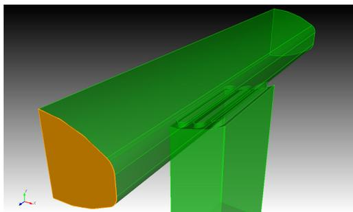
Figure 5: CUBIT half model for the pumping slots.
