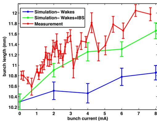
Figure 3: Simulated bunch length as a function of current, compared with a streak camera measurement.
