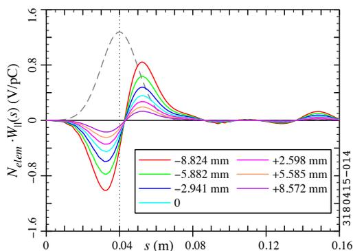
Figure 6: Longitudinal wake of the pumping slots for different vertical displacements.
