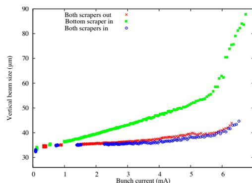
Figure 8: Vertical beam size vs current, with different scraper configurations. There is a strong beam size blowup when only the bottom scraper is inserted.
