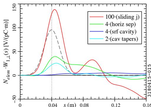
Figure 4: Transverse vertical wakes calculated with T3P for a 10 mm bunch, scaled by the number of elements in CESR.
