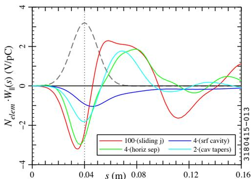
Figure 2: Longitudinal wakes calculated by T3P for a 10 mm bunch, scaled by the number of elements in CESR. The dashed grey line represents the bunch distribution.
