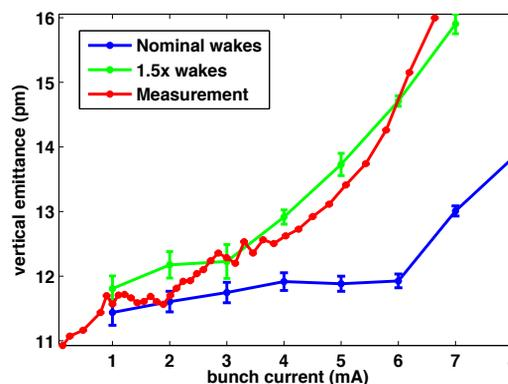
Figure 7: Vertical emittance in tracking simulation, with transverse monopole wakes included, compared to a measurement made with an x-ray beam size monitor [15].
