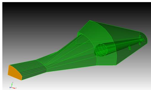
Figure 1: CUBIT quarter model of the horizontal separator.
