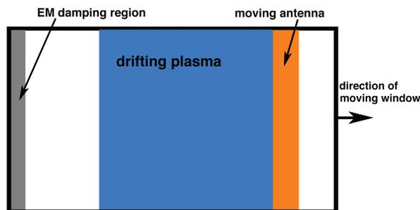
Figure 1: Cartoon of simulation setups for the LWFA simulation in the Lorentz boosted frame. The plasma, and moving antenna are drifting from left to right, in the same direction as the moving window.
