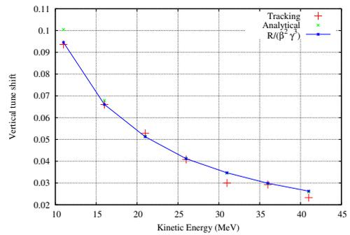
Figure 4: Tune shift as a function of the energy in the KURRI scaling FFAG. Good agreement between the analytical formula 9 and the tracking results is shown. (The perveance taken here is  $Q = 6.4 \times 10^{-8}$ ).
