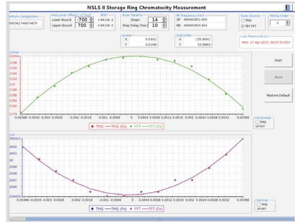
Figure 2: Measurement of chromaticity with the NSLS-II TbT tune measurement system:  $\xi_x = 0.03, \xi_y = 0.01, \xi_{2x} = -135.8, \xi_{2y} = 52.7$ .
