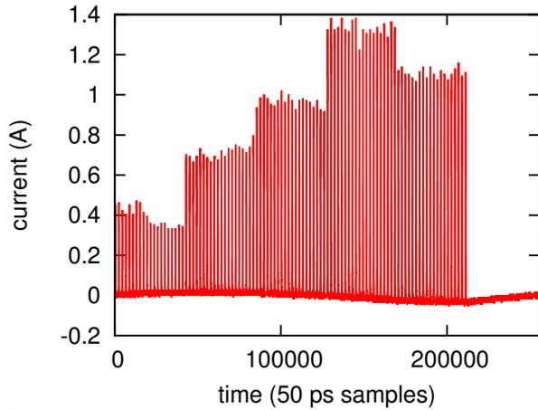
Figure 1: Wall current monitor data for the blue ring at the beginning of the experiment.
