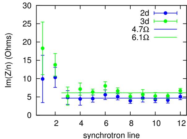
Figure 5: Measured  $Z/n$  with one sigma error bars in yellow for 12 synchrotron lines. The averages for lines 3 through 12 are shown.
