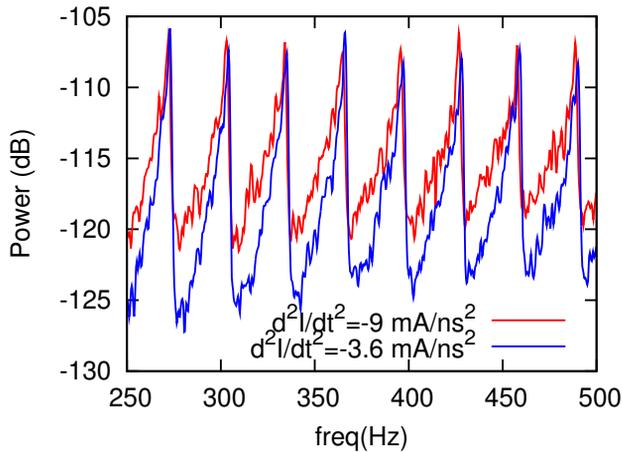
Figure 2: Yellow longitudinal Schottky spectra for synchrotron lines 5 through 8 at two different intensities.
