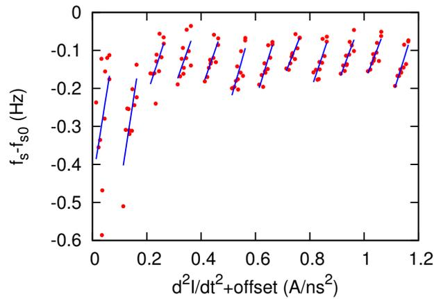
Figure 3: Yellow synchrotron frequency versus  $d^2I/dt^2$  in the center of the bunch for first 12 synchrotron lines. No drift with time was included.
