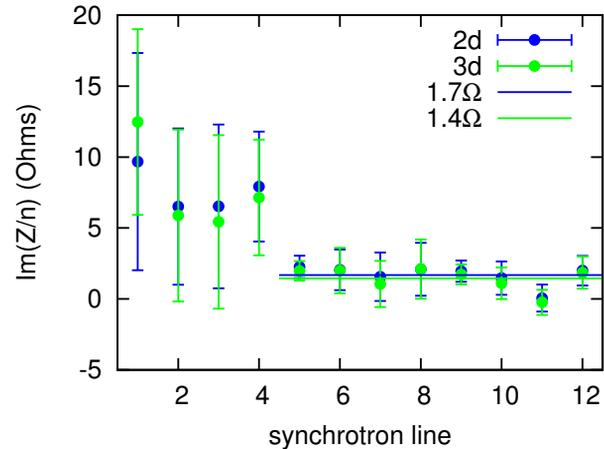
Figure 4: Measured  $Z/n$  with one sigma error bars in blue for 12 synchrotron lines. The averages for lines 5 through 12 are shown.
