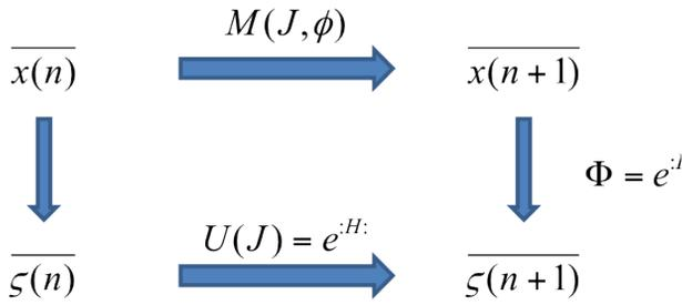
Figure 2: A schematic drawing showing the process of normal forming the one turn map of a storage ring, where an action-angle dependant one turn map gets transformed into an action only dependance map.
