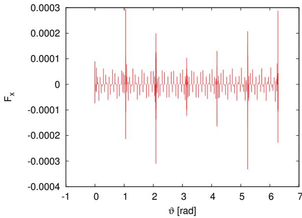
Figure 1: An example of  $(1 + G\gamma) \frac{B_x}{(B\rho)_0}$  seen by a test particle with  $G\gamma = 62.33$ .
