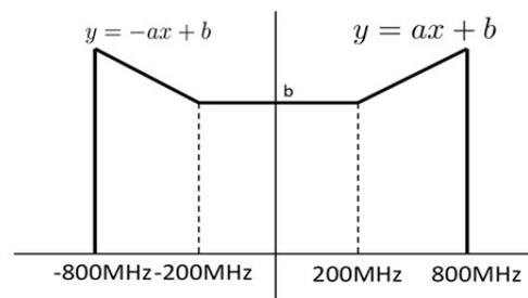
Figure 10: Desired frequency response for BPM.
