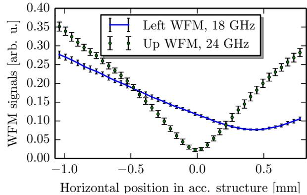
Figure 2: A scan over horizontal positions. The 'Left' signal filtered at 18 GHz and the 'Up' signal filtered at 24 GHz are shown.
