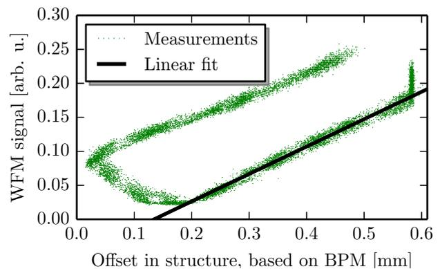
Figure 4: Left WFM signal at 24 GHz as a function of the vertical beam position (green). A linear fit was performed on a portion of the data.
