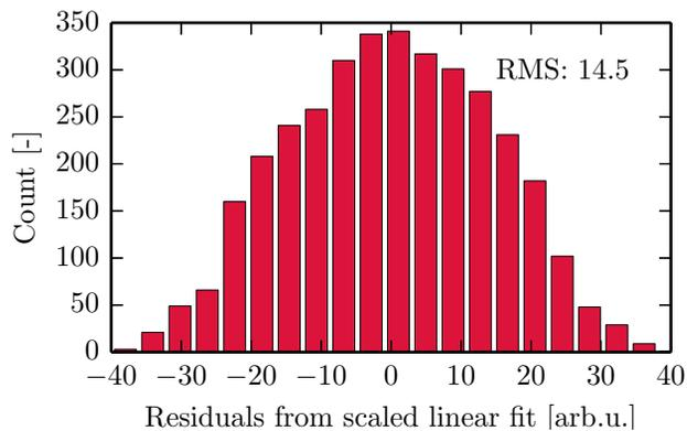
Figure 5: Residuals of the linear fit from Fig. 4, scaled so that the average WFM and BPM measurements give the same value. The RMS of the residuals of 14.5 then gives a merit for the precision.
