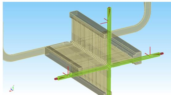
Figure 1: The internal geometry of a TD26 structure except for the first coupling cell. The WFM waveguides are shown in green and the pickup antennas in red.
