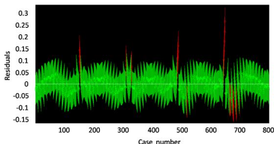
Figure 2: Residual plot of  $s_{21}$  term of gap's transfer matrix.
