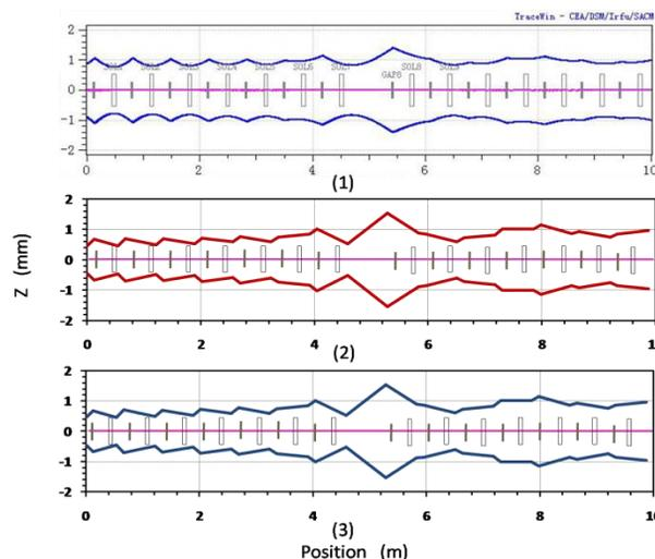
Figure 3: The envelopes of TRACEWIN (the upper picture), the broken line graph of beta in MATLAB (the middle picture) and the broken line graph of beta by hardware simulation (the down picture).
