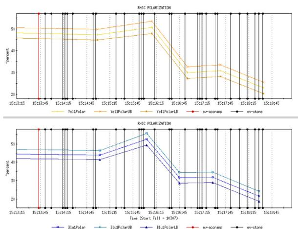
Figure 4: Polarization measurements on ramp. The vertical lines are step stones on the ramp to define energy, optical parameters. The dense lines usually indicate strong depolarizing resonance locations.
