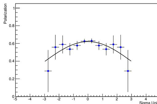
Figure 2: The polarization profile from a single measurement at store. The horizontal axis is in unit of beam size sigma.
