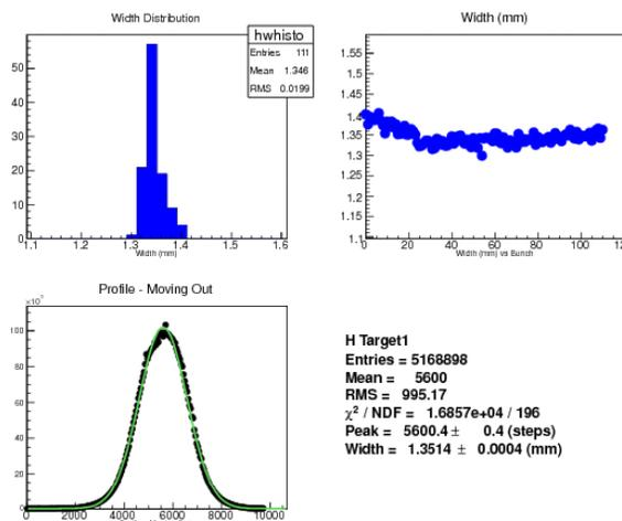
Figure 5: Emittance measurement in Blue ring. The profile at left bottom is for all 111 bunches, the beam width on the right top is for all individual bunches.
