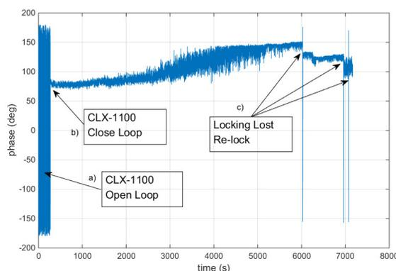
Figure 5: Result of laser phase measurement: a) CLX-1100 open-loop, b) CLX-1100 closed-loop, c) Phase Locking Lost due to picomotor movement.
