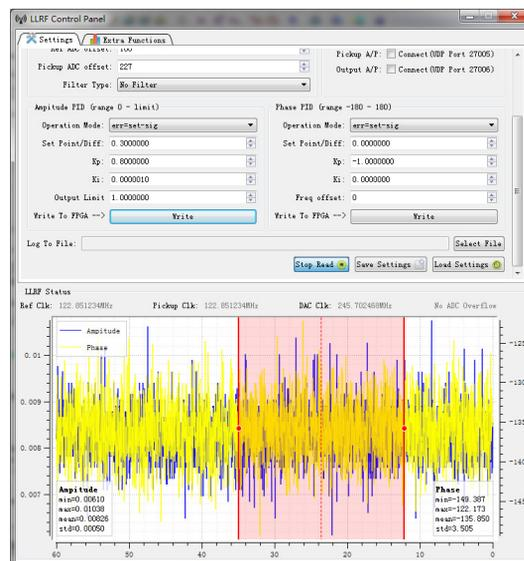
Figure 8: Control Interface of LLRF.
