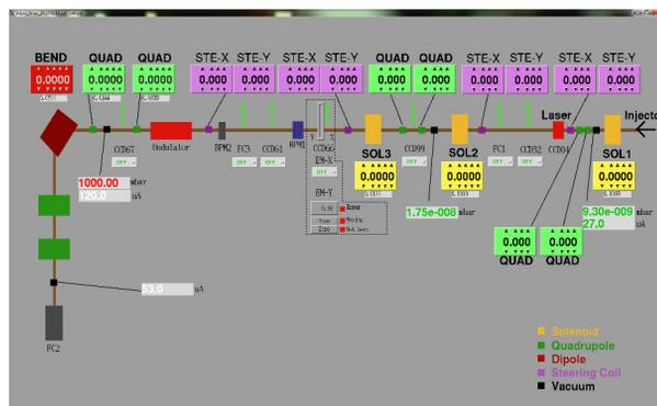
Figure 4: MEDM screen of the beamline control.
