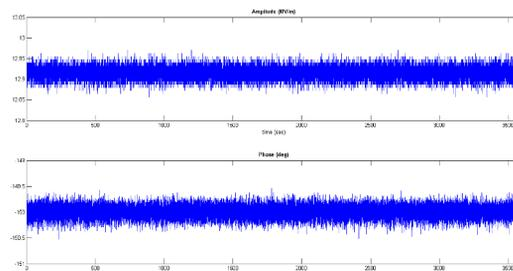
Figure 7: Cavity amplitude (up) and phase (below) plot at 12.9MV/m without beam-loaded.
