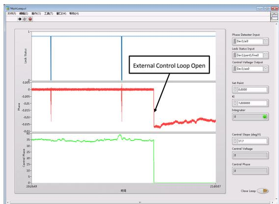
Figure 6: Control Screen of External Laser Phase Lock. Blue curve: CLX-1100 Lock status. Red curve: Phase error signal. Green curve: phase correction signal
