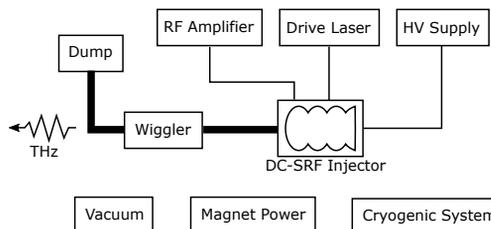
Figure 1: DC-SRF injector THz wiggler radiation experiment layout.
