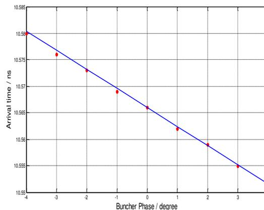
Figure 4: arrival time versus buncher phase.
