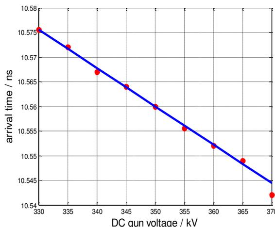
Figure 1: arrival time vs DC gun voltage.
