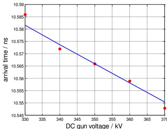
Figure 3: arrival time voltage versus DC voltage.
