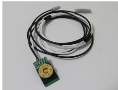
Figure 3: Prototype of CVD diamond BLM detector.
