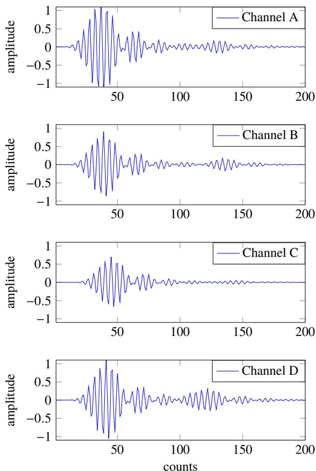
Figure 3: Signals were calculated with the following parameters:  $K_x = K_y = 1$ ,  $(x_0, y_0) = (0.2, 0.1)$ , and other time lags and coefficients were randomly chosen at exaggerated intervals to amplify the measurement errors.
