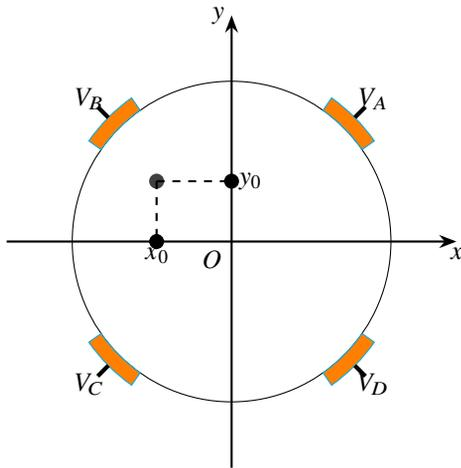
Figure 1: The 4-pickup BPM layout.
