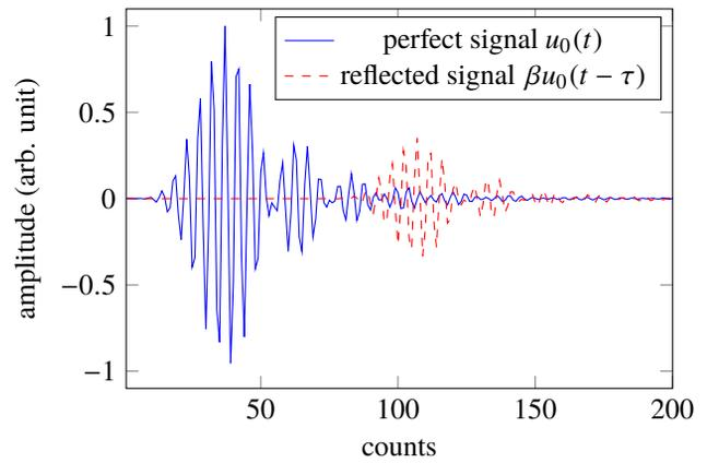
Figure 2: Samples from real measurements and its shifted, scaled reflection signal.
