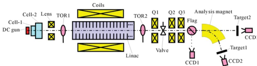
Figure 1: Layout of the HUST THz-FEL LINAC.
