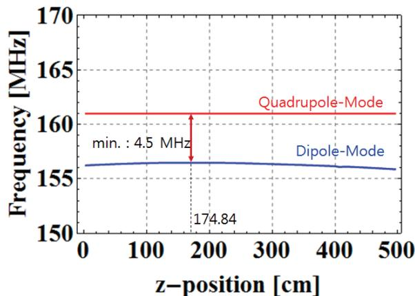
Figure 5: The adjacent mode frequency.
