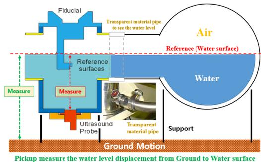
Figure 2: Half-filled water pipe.
