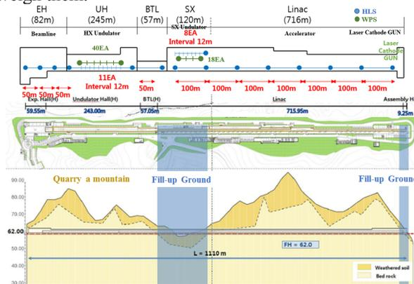
Figure 8: The geography of PAL-XFEL and the installation location for HLS.
