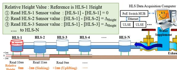
Figure 4: HLS relative measurement (methods for routine measurement and displaying values).
