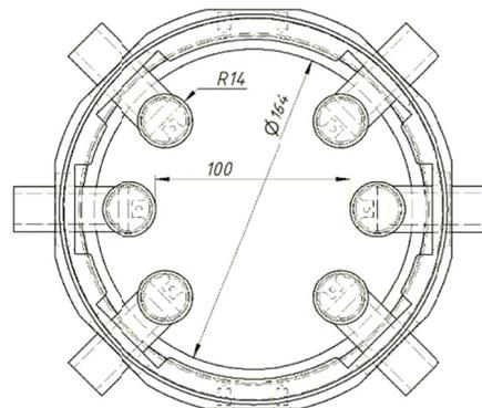
Figure 9: The kicker actual design (all dimensions are in mm).
