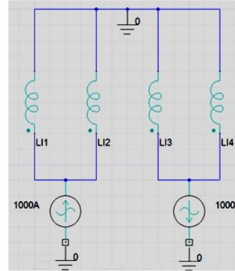
Figure 4: Simplified equivalent electrical circuit of the magnet.
