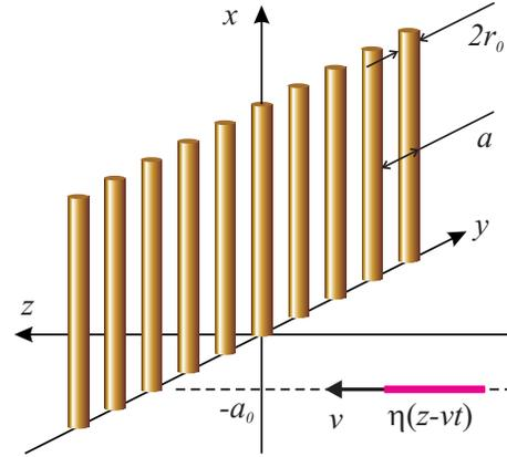
Figure 1: Bunch passing by the edge of a grid structure.
