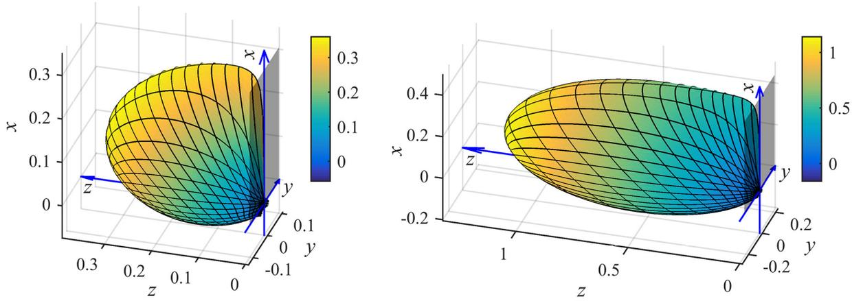
Figure 3: Spectral angular density of energy radiated by a charge moving orthogonally to semi-infinite wire grid at small distance from the edge. Parameters of the grid: wires are made of copper ( $\sigma_e = 5.8 \times 10^7$  S/m),  $a = 10$  mm,  $r_0 = 1$  mm; frequency  $\omega = \pi c/(5a)$ , bunch velocity  $\beta = 0.7$  for the left plot and  $\beta = 0.9$  for the right plot. Radiation density is normalized on  $4|\tilde{\eta}|^2/c$ .
