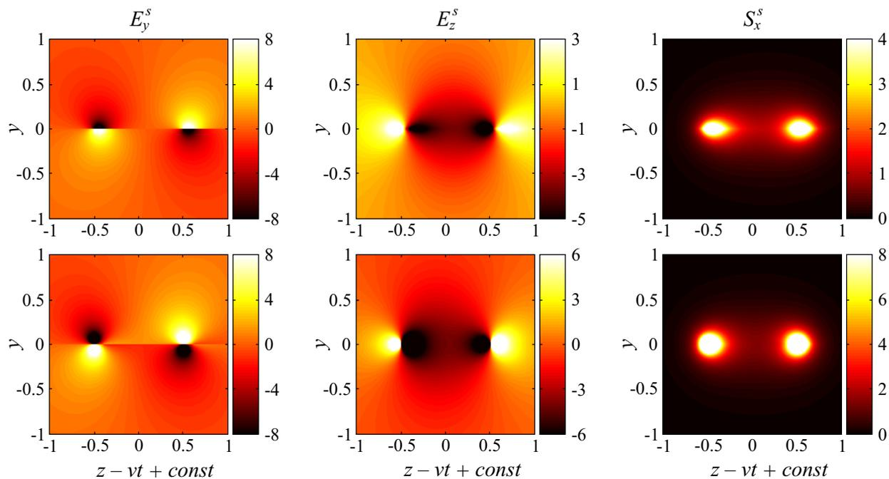
Figure 5: The field components and the energy flow density of the surface wave generated by rectangular moving along the edge of semi-infinite wire grid (Fig. 2) in the plane  $x = x_0 = const > 0$ ,  $\zeta = z - vt$ . Wires are PEC, Gaussian units are used. Bunch length is 1 cm, the charge is  $q = +1$  esu;  $a_0 = 0$  cm and  $b_0 = 0.1$  cm (the first row),  $a_0 = 0.1$  cm and  $b_0 = 0$  cm (the second row),  $\tilde{\kappa} = 0$ ;  $\beta = 1$ .
