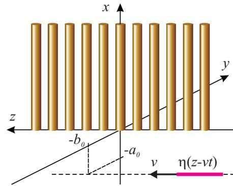
Figure 2: Bunch moving along the edge of a grid structure.
