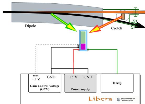
Figure 8: Proposed acquisition electronics including power supply and gain control for the PMT.
