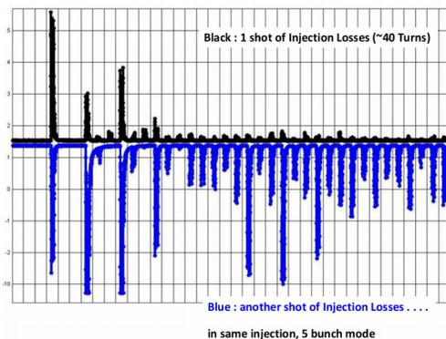
Figure 4: Two injection shots, showing different losses in first tens of turns.
