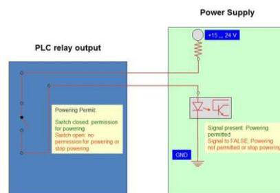
Figure 2: “Powering Permit/Stop Powering” signal exchange.
