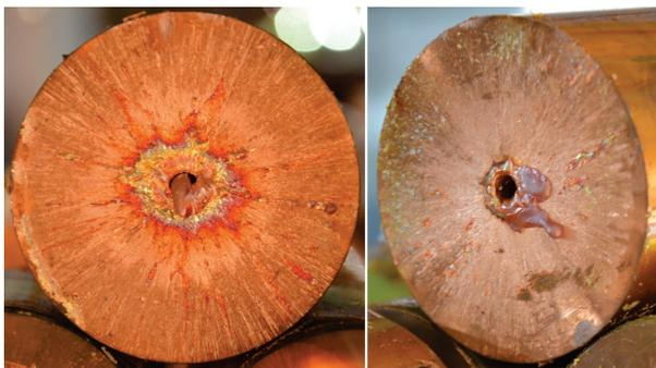
Figure 3: Front (left) and back (right) faces of the third cylinder of target 3. Re-solidified copper splashes and the hole generated by the beam is visible.
