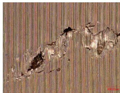
Figure 7: Micro-Cavity at  $z = 85$  cm in Target 3. The area is located on the beam axis with a surface of  $\sim 1.5$   $\text{mm}^2$ .
